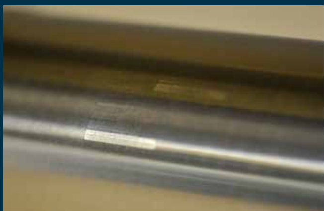
g) Indicator: Facets occur parallel to the workpiece axis (partial or over the entire circumference)
